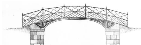
'Wrought and cast iron arch bridge'
